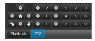
When a camera has PTZ capabilities the PTZ tab will be clickable. Clicking on this tab will bring up the interface to the left.
